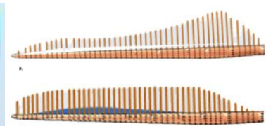
Comparison of total thrust at 0° and at 3.5° for R.2 LLJs
